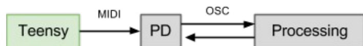
Figure 52. First communication setup. Teensy transmits through MIDI to pd-extended. Pd-extended and processing communicate via OSC messages.
